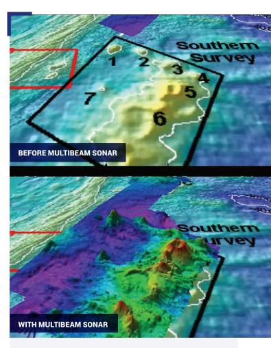
The top image shows what we previously knew about the seafloor terrain in the Southern Mariana region from satellite altimetry data. The bottom image includes an overlay of the information provided by *Okeanos Explorer's* EM302 Multibeam System. *Image courtesy of NOAA OER*.
